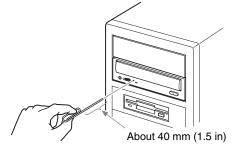
Depending on the product you are using, the Emergency Eject Hole may be in a different location than illustrated above.
